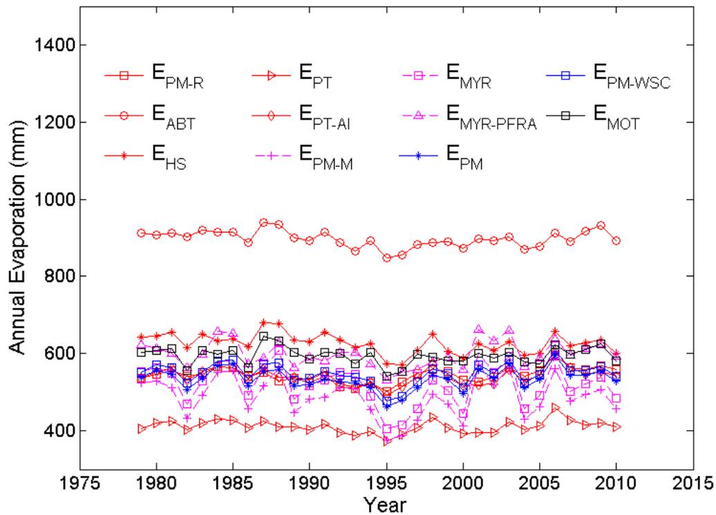
Figure 5: Comparison of annual lake evaporation calculated from various methods at Brazeau Reservoir.
