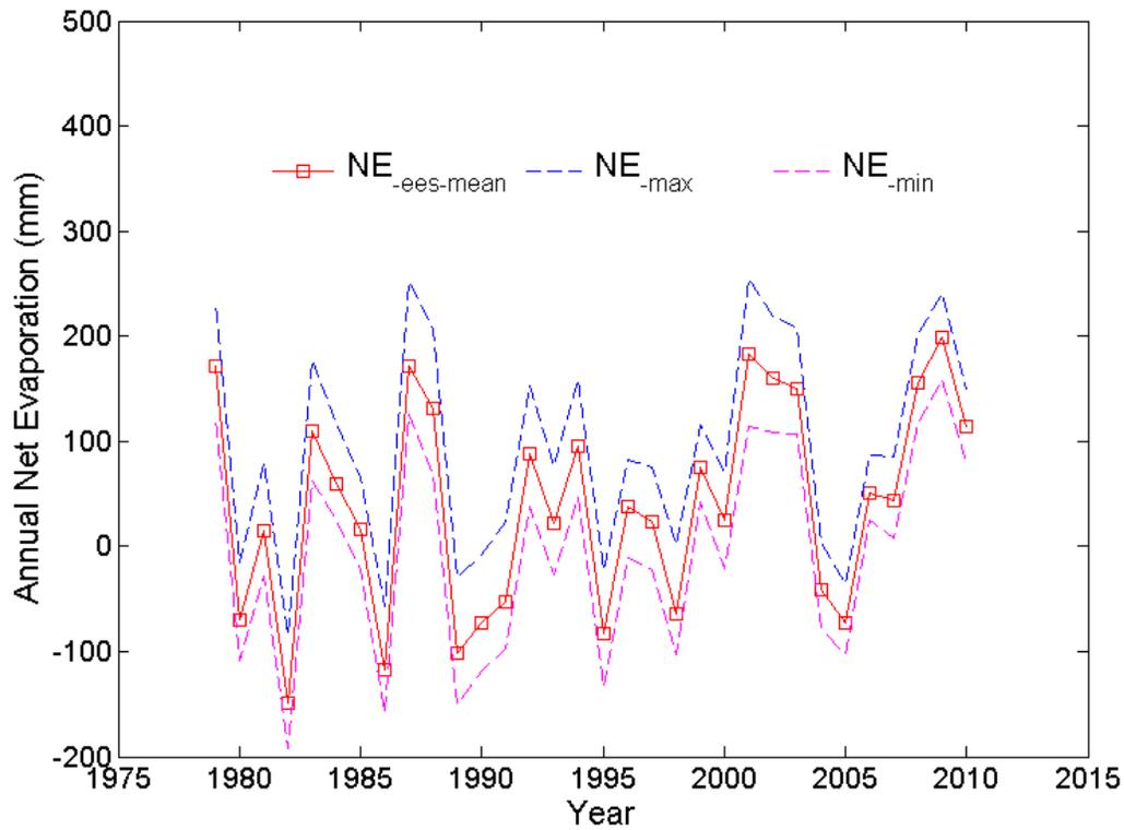
Figure 14: The minimum, maximum, and mean of annual net lake evaporation of Brazeau Reservoir.
